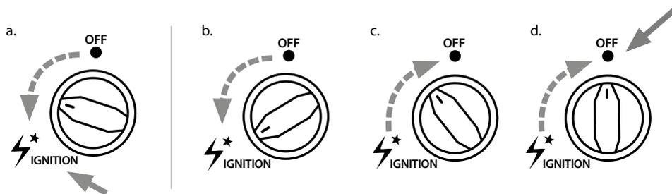
a.) Ignite the burner by turning the control knob anticlockwise towards IGNITION until you hear a click. The clicking sound is the ignition and the burner should now ignite.
